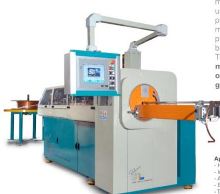
The SILVER series pipe bending machines, with feeding from coil, are use to bend light alloy and other alloy pipes. The "BRUSHLESS" electric motors, installed on the machines, provide the three basic movements: bending, rotation and feeding. They give these advantages: no maintenance, noise reduction, optimization of movements. greater cleanliness, reduced power consumption. The orbital
