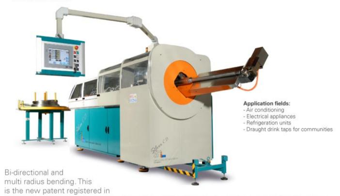
2002. The system for moving the dies offers automatic changing of the bend radii on the same pipe, offering also right and left rotation. The SILVER 2 CD, with its six controlled axes, stands at the top of the world manufacturers of pipe benders without mandrel with integrated orbital cut.
